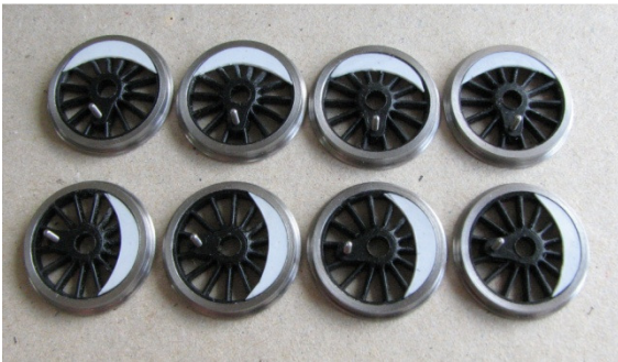
Gibson wheels fitted with crankpins and balance weights.
