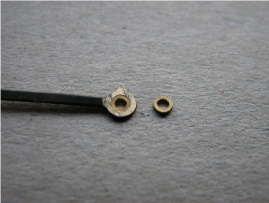
Bush in rod ready for soldering.
